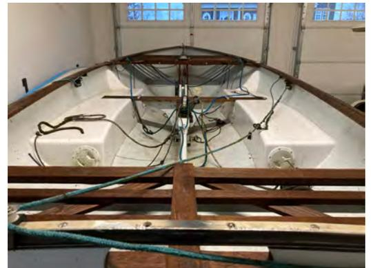
We removed all the existing hardware and cataloged each piece. Once that was completed we started sanding down the teak and then washed down the interior and exterior of the hull.
