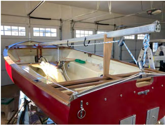
Having completed the hull, we attached all the running rigging and lines connected with operating the boat.
