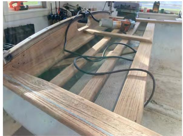
We then proceeded to put three coats of teak oil on all the wood with a slight sanding in between coats. In addition we put our first coat of Hatteras Beige on the interior. We allowed one week for that coat to dry and then applied the second coat.
